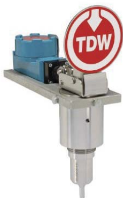
Figure 1. The TDW PIG-SIG® V with flag and electrical indicator. The plug and indicator assemblies interact via opposing magnets.
