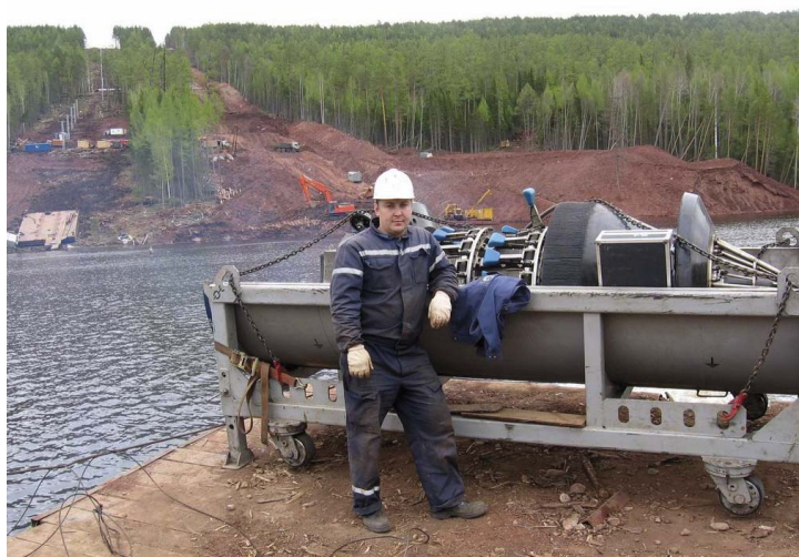
Figure 1. Preparation of the geometry tool at an underwater crossing of the Ust-Ilimsk reservoir. Pictured is P. Sherman, a technician of the profilometry department of the Ufa branch of Transneft Diascan.
