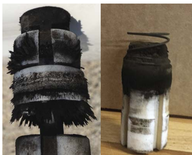
Figure 2. Left: A magnet equipped with a filter pack. Right: A magnet without one. The filter pack provided a barrier against ferrous debris building up on the magnet itself. Without a filter pack, ferrous debris on and around the magnet kept the pig passage indicator from operating as designed.
