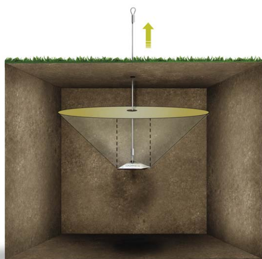
Figure 3. Typical frustum of soil in granular soil.
